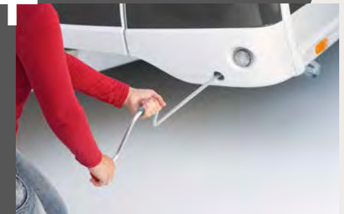
Crank insertion aid for convenient operation of the crank supports
