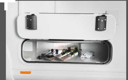
Frost-proof – thanks to the heated double floor with plenty of storage space and through-loading facility
