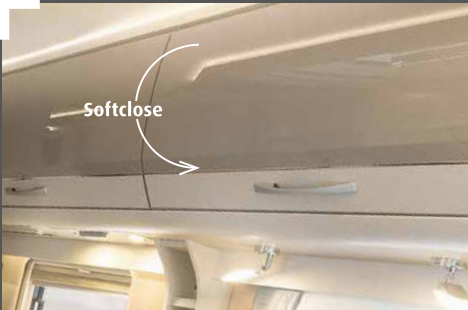
The high-gloss overhead lockers are equipped with a soft-close function and are indirectly illuminated
