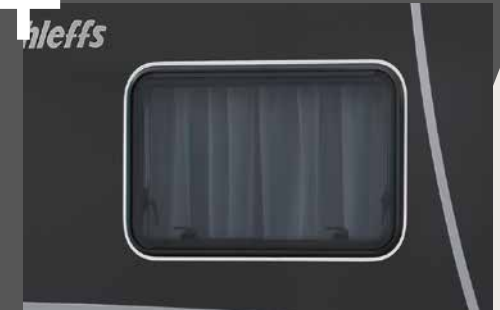
Well-insulated and secure: automotive flush-fitting windows
