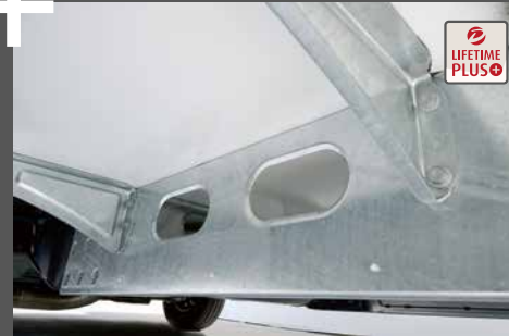
Dethleffs Lifetime-Plus: GRP-clad, wood-free underfloor, side walls with PU strips and XPS insulation
