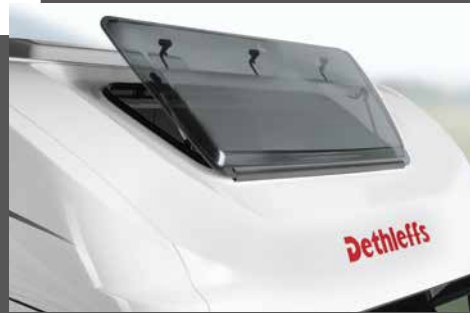
Openable window in the cab hood for more light and air inside the vehicle
