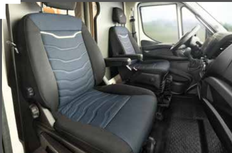
Ergonomic captain seats, multiadjustable, with seat heating and hydraulic suspension
