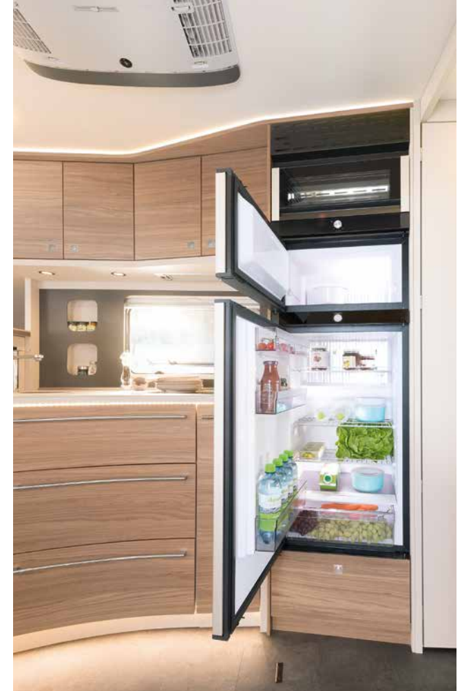
The large drawers include an electric central locking system and are locked automatically when the engine is started.
