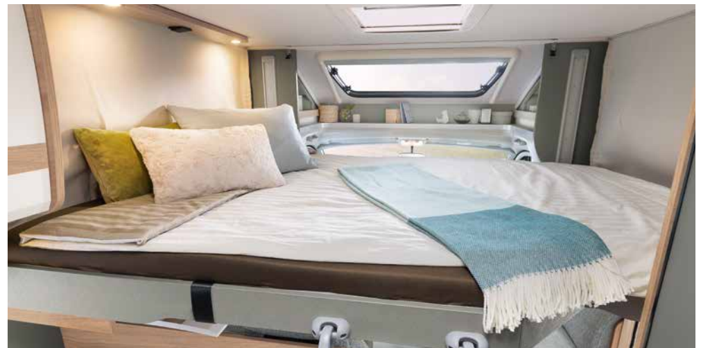
Electrically operated two-person pull-down bed above the seating lounge (option)
