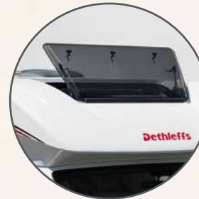
Large opening skylight in the cab hood
